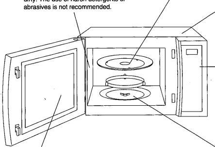
Roller Ring and oven cavity floor:
